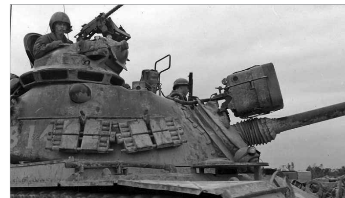
An M48A3 Patton tank in Vietnam: 1stLt Harris Himes' platoon operated five of these armored giants. Note the TC's cupola
